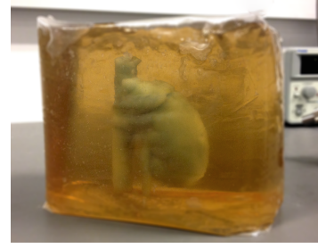
Fig. 4. Human-kidney phantom immersed in a background water-based gel.
